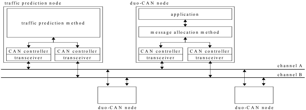
Fig. 1 Structure of CAN network system with dual communication channels
