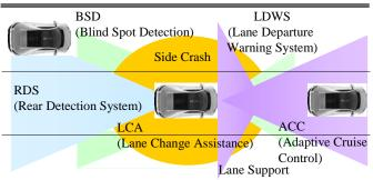
Figure 1: Advanced Driver Assistance System for intelligent vehicles.
